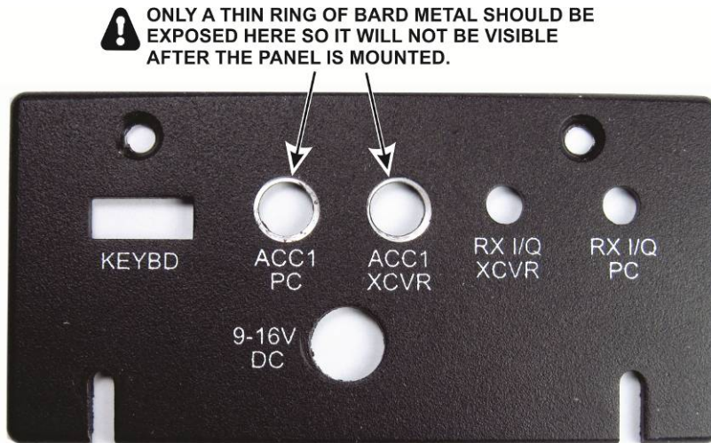
Figure 37. Checking the Grounding Surface on the ACC1 PC and XVCVR Connector Openings.
